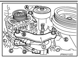
12. Remove alternator assembly downward from the vehicle.
