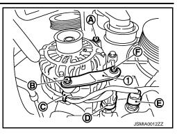
12. Remove alternator assembly downward from the vehicle.
