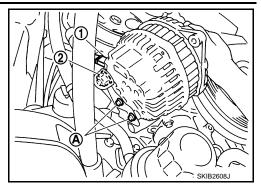
13. Remove alternator assembly downward from the vehicle.
